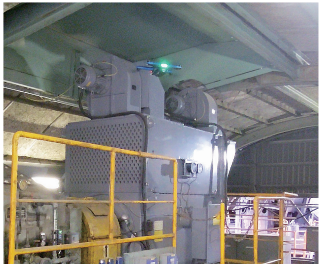
Equipment inspection by drone (Kumagaya Plant)
