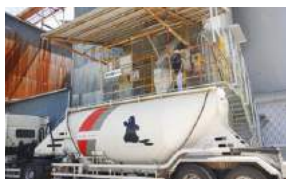
Hatchway, safety blocks and safety full body harness
