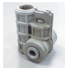
Casting mold for T-shape pipe
