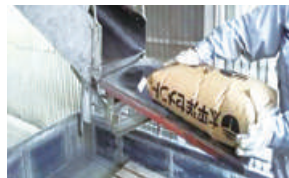
Measure to prevent being dragged into equipment at the Yokohama-Minami service station
