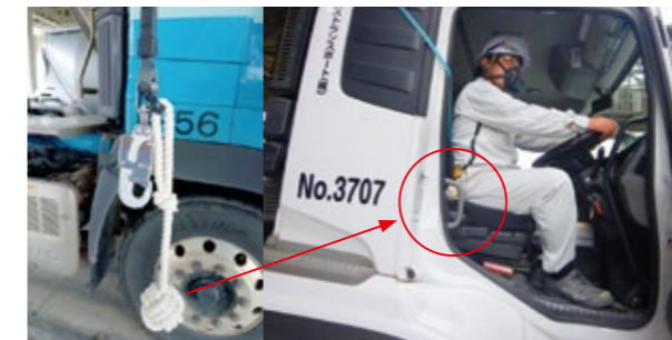
Ball-shaped object attached to the safety block → The person will feel discomfort when getting in the vehicle and realize they have forgotten to remove the fall prevention device
