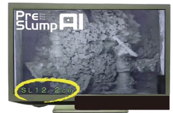
Monitor display of the post-mix slump prediction system "PreSLump AI"
