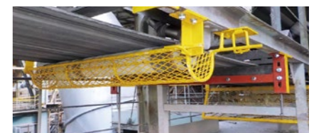
Safety cover for self-aligning return roller Registration No.: 03235767 (February 3, 2022)
