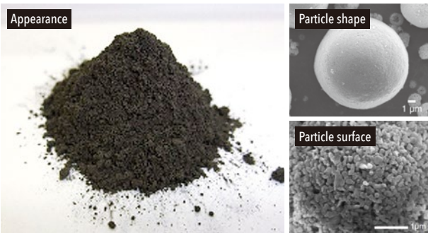
"Nanolithia," a cathode material for lithium-ion batteries
