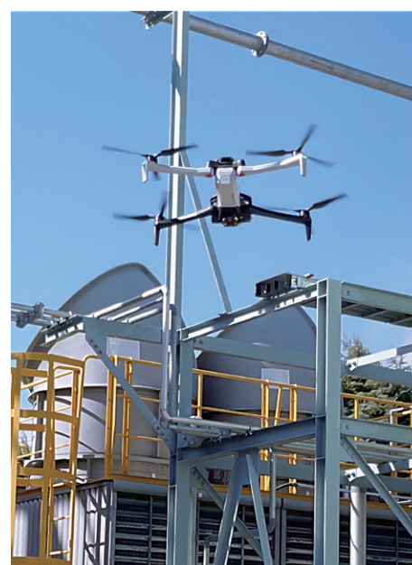
Equipment inspection using drones
