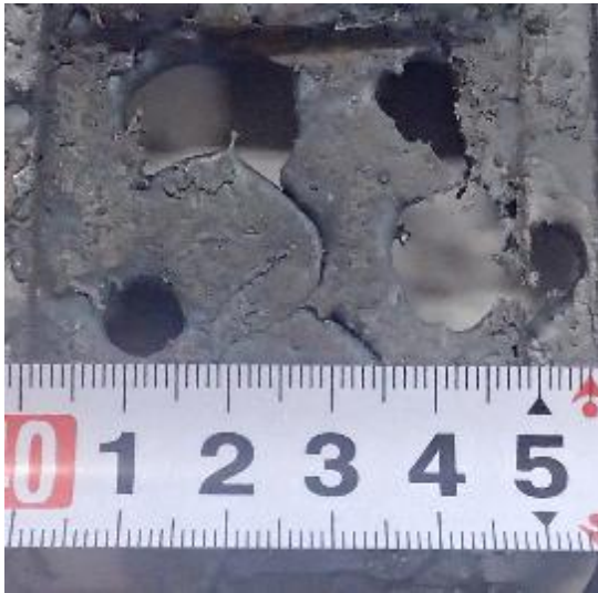
A casting with blow holes
