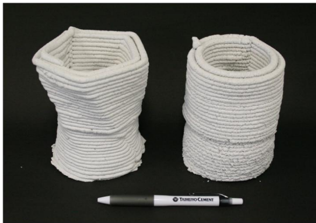
Photo 2 The first test models in Japan manufactured by the said technology
