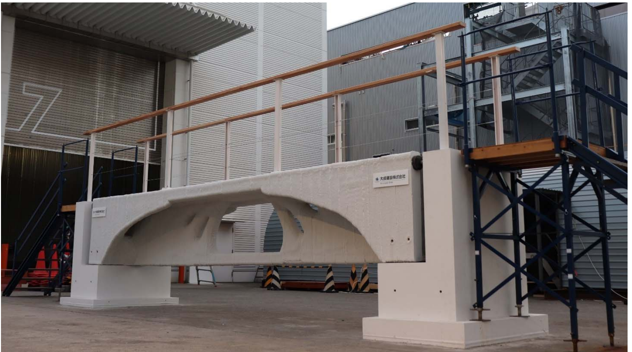
(Photo 2) A “bridge” strong enough to support people (length: 6m)
