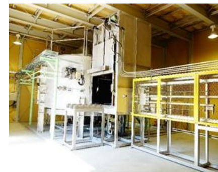
Facility for torrefied recycling of lithium batteries (Tsuruga Cement Co., Ltd.)
