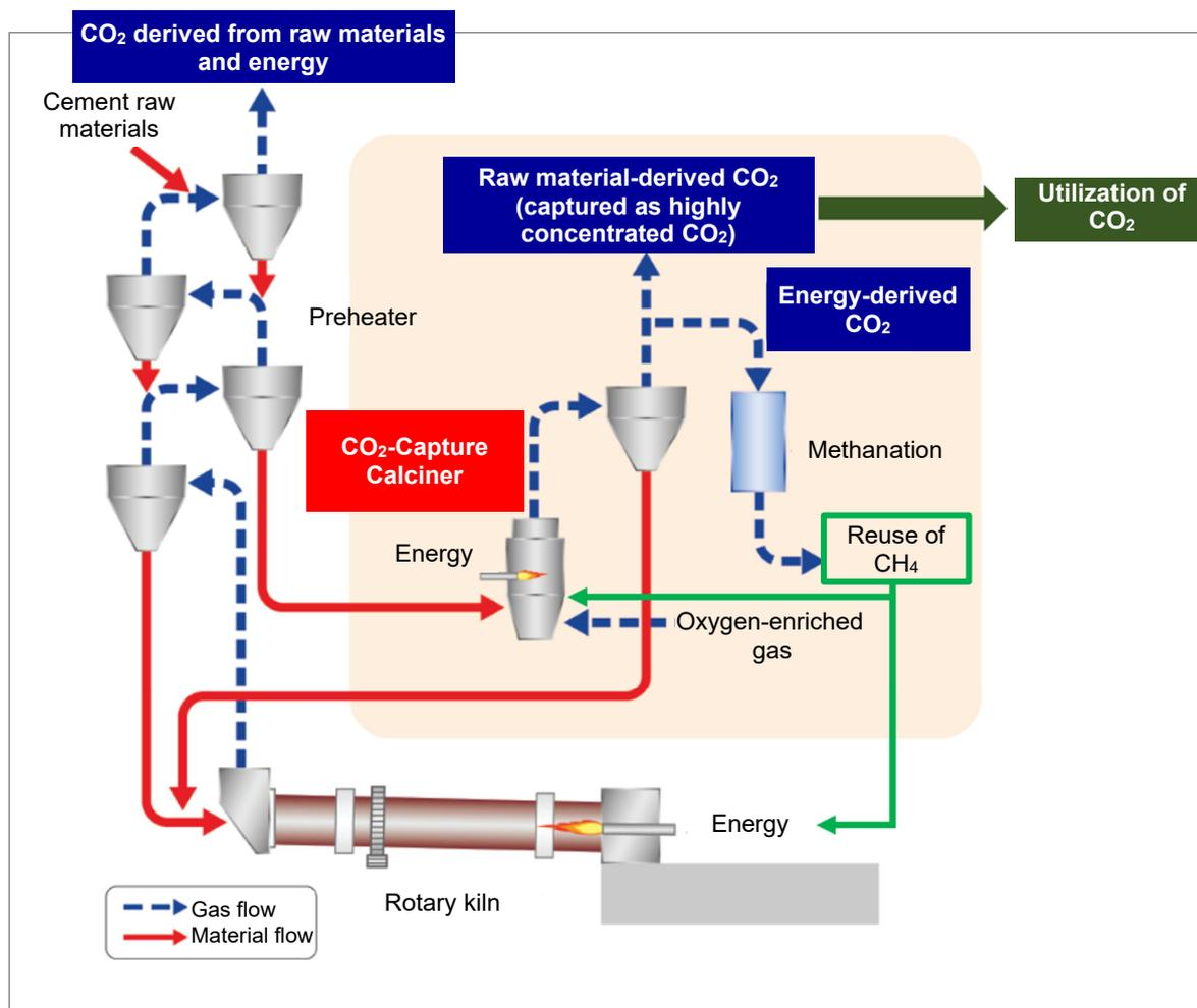
Concept of the cement production process that captures CO<sub>2</sub>
