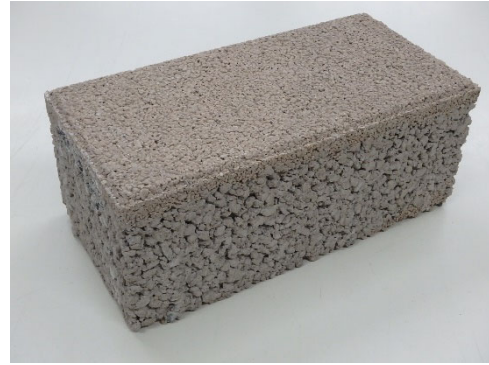
Photo 2. Interlocking block made of CARBOFIX cement
