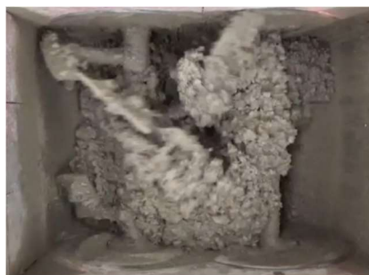
Fresh concrete during mixing
