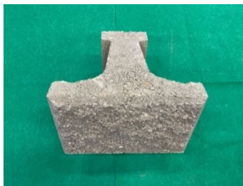
Photo 1: A building block made of CARBOFIX cement
