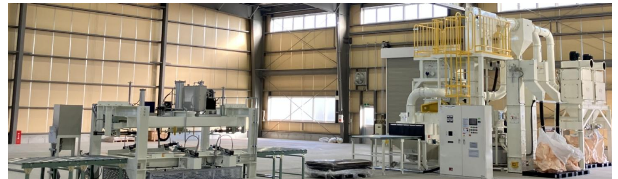
Waste solar panel treatment equipment at Nacode Co., Ltd. (100% owned subsidiary of the Company)
