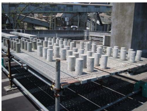
Fig. 1 Outdoor exposure test (暴露場の景観及び暴露状況)
