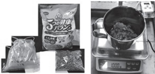
Fig.2 Materials under test (cement raw meal and simulated sewage sludge made from dog foods blended with water) (供試原料 (ドッグフードと水を混合した模擬汚泥とセメント原料))
