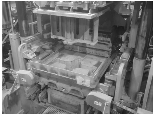
Fig.7 Molding situation with pressure vibration molding machine (加圧振動成形機での成形状況)
