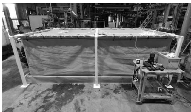
Fig.9 Exterior view of portable carbonation curing equipment (簡易炭酸化養生設備の外観)
