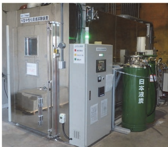
Fig.2 Carbonation curing chamber (炭酸化養生槽)
